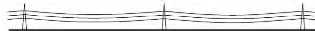
Spans normally vary from approximately 250 to 400 metres. Minimum safely clearances must be maintained under the conductors. The clearances are greater over roads.
