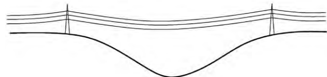
Valleys allow the use of long spans but excessive spans may require the use of 30° angle towers at either end.
